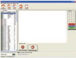
Paging Software Main Screen allows communications to be sent direct to pagers from a PC on the stadium LAN
